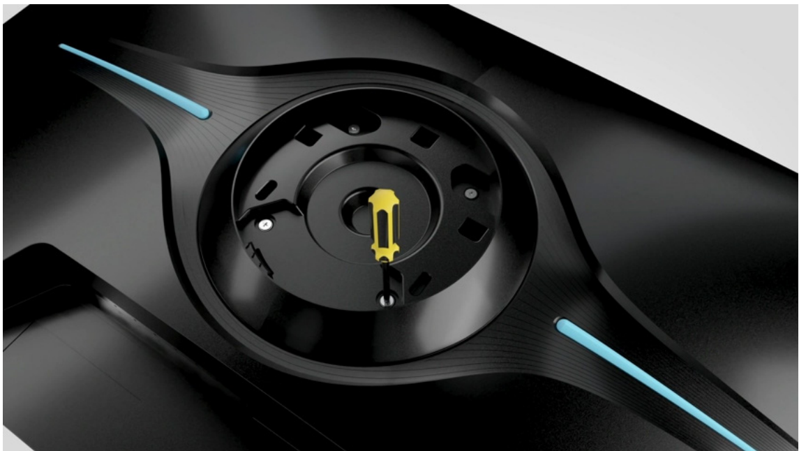
Remove the retaining screws for the back cover
